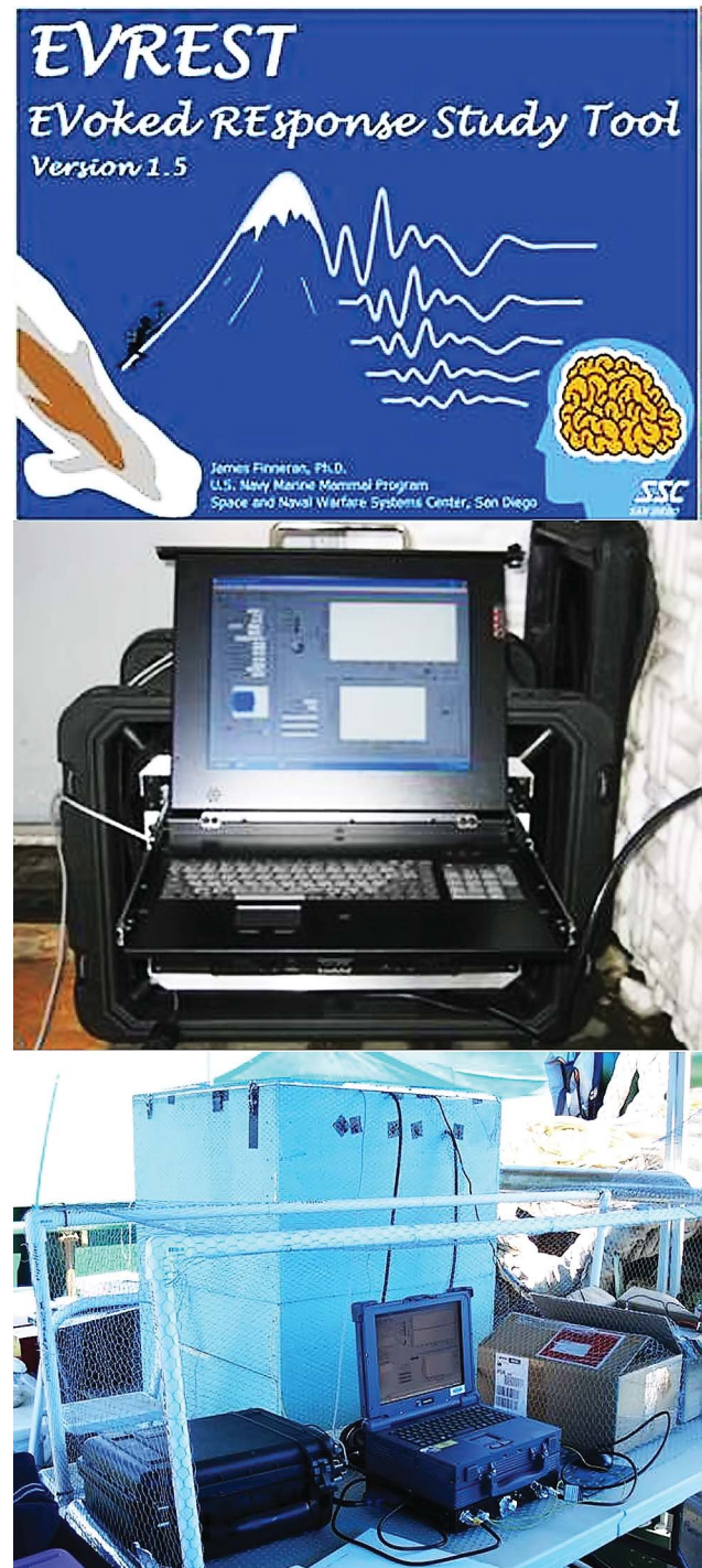
Fig. 5. Field portable system developed at Space and Naval Warfare Systems Center (SSC) San Diego consisting of bioamp (in Pelican case, bottom photo, shown with system running onboard a ship), ruggedized computer with data acquisition hardware, and Evoked Response Study Tool (EVREST) software developed by J. J. Finneran for generating sound stimulus signal, recording and storing auditory evoked potentials (AEPs), and analyzing data.
