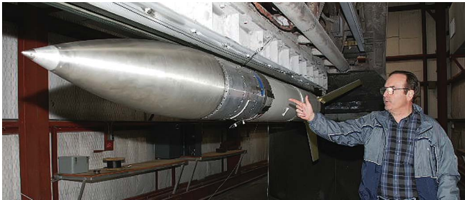
Fig. 8. Orion rocket attached to launch rail.
